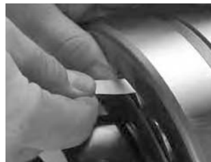
Fig. 91. Measure RIC before installation.
