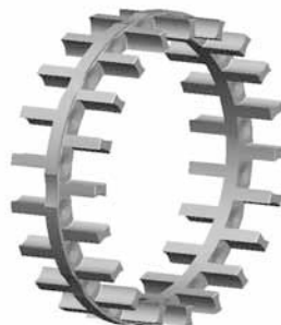
Fig. 49. One-piece finger-type cage.
